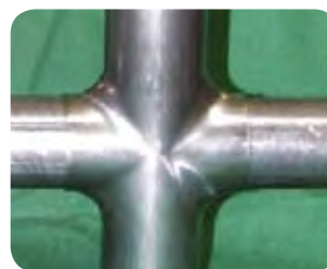
1.4003 hydroformed welded tube.
