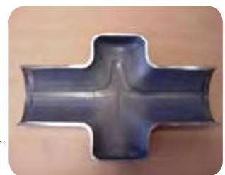
Deformation of the weld (1.4003).
