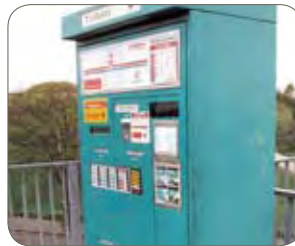
Grade 1.4003/410, painted (15 years in service), SASSDA, UK
