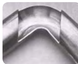
Bending of 430T welded tube.
