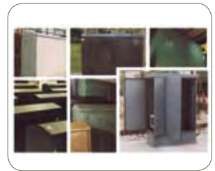
Grade 1.4003/410, painted (15 years in service), SASSDA, South Africa
