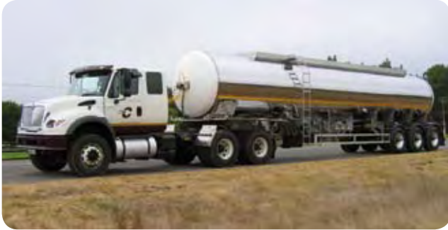
Milk tanker, cladding in grade 430, S. Africa.
