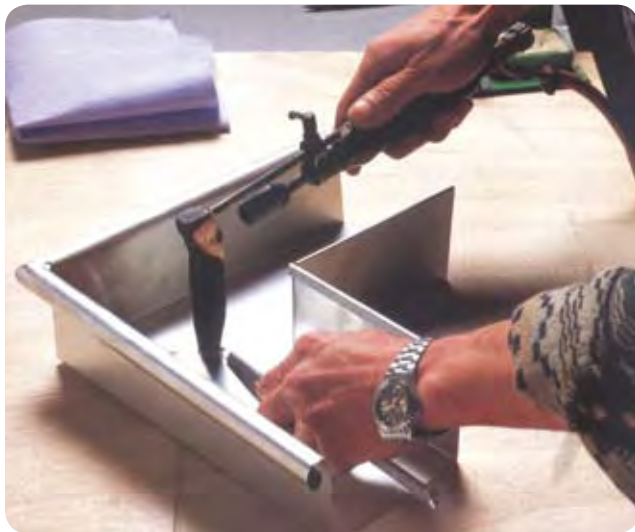
Soldering a gutter, tin-coated grade 430Ti.
