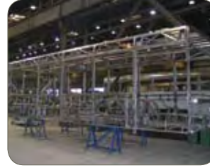
Grade 1.4003 welded tubes and panel, Solaris Bus & Coach Co. Poland
