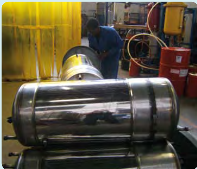
Welded tank, grade 441, S. Africa.
