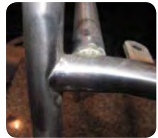
Brazing welded tubes, grade 441.
